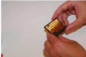
*A photograph of the world's first transceiver integrated on a single chip that operates at 60-GHz on the CMOS process. It allows wireless transfer of audio and video data at up to 5 gigabits per second, ten times the current maximum wireless transfer rate, at low cost.*
