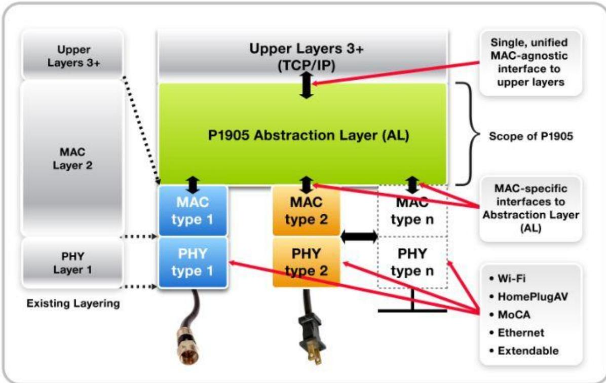
Fig.3: P1905.1 brings seamless bridging to the home network by introducing a software layer between layers 2 and 3 that abstracts the particular operating details of each interface in use. P1905.1 thus provides quality of service (QoS), device configuration, secure connections, among other advanced network management features
