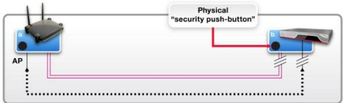
Fig. 5: P1905.1-compatible devices are configured with a single button-press to avoid the complexity of password entry. P1905.1 also enables consistent password and authentication procedures to support legacy devices.
