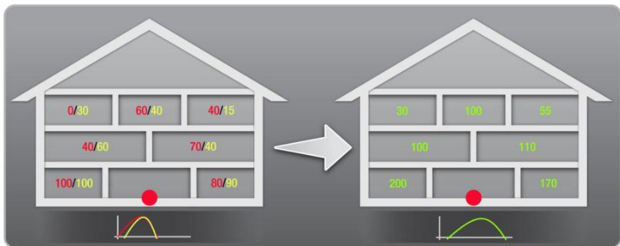
Fig. 2: The use of multiple connectivity technologies provides redundant coverage in key rooms in the home so that the quality of content can be maintained regardless of changing operating conditions. The numbers in magenta in the left half of the figure signify the data throughputs in different rooms if only one technology per room is used; the yellow figures indicate the throughputs only with a different technology. The green numbers on the right side of the figure show the effective throughput when both technologies are used simultaneously. The red ball is the location in the home where broadband entry point is located. All measurements are in Mbps
