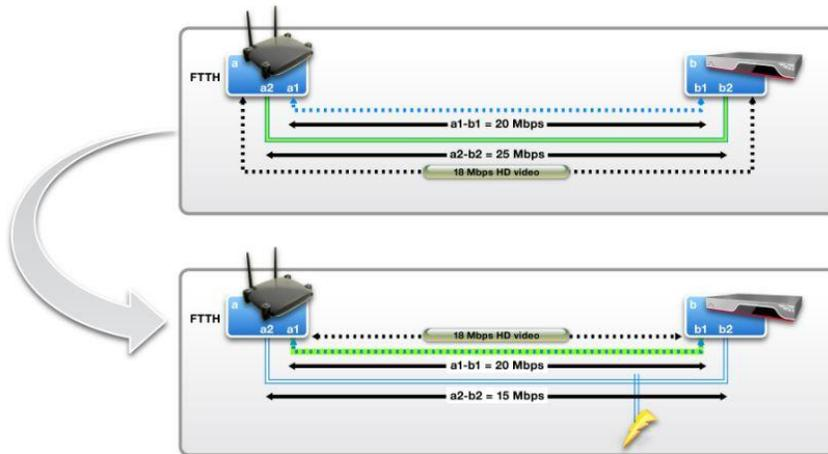
Fig. 4: P1905.1 maintains content quality and reliable service through the use of path selection to resolve common network issues such as congestion and interference.
