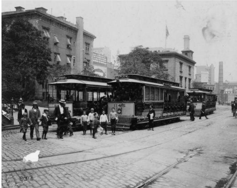
Figure 13 - An open car and a semi-enclosed vehicle wait at Park Rowe before takeoff in 1898. Each car carried 60 passengers. Courtesy of the Schenectady Museum, General Electric Collection.
