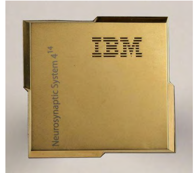
IBM's neurosynaptic processor, 1 M Neurons and 256 M Synapses
