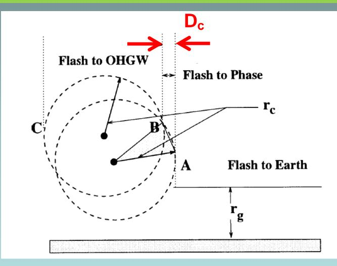
**D**<sub>c</sub> - Exposure Distance for a shielding failure
