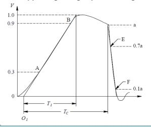
Front-chopped Lightning Impulse Voltage
