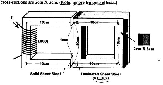
Draw the 'electric equivalent' circuit. Label the elements including the source, NI, and the air gap(s).
