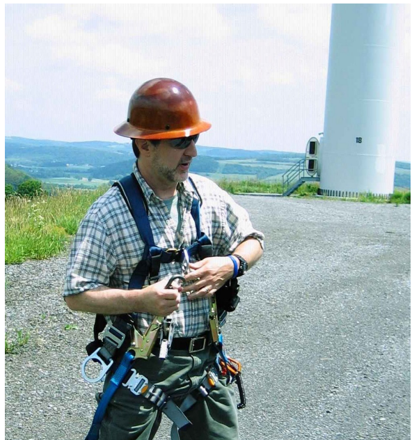
Kevin Wigell shown demonstrating the harness used when climbing the wind turbine for maintenance.
