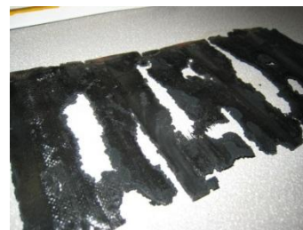
Photo 4. Side packing almost completely eaten away by vibration sparking.
