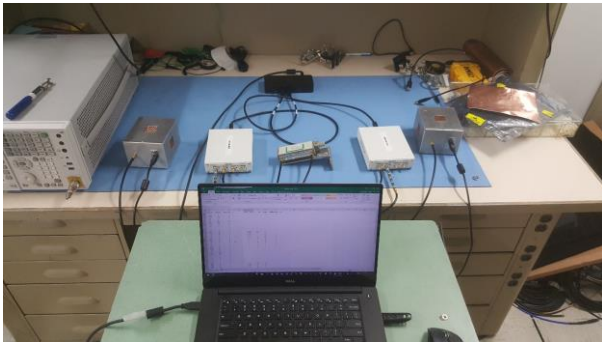
Frequency agile OFDM test capability – enables wireless link testing in non-standard bands (e.g. 4.3 GHz)
