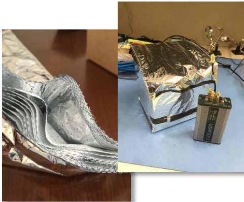
Signal attenuation measurement through multi-layer insulation
