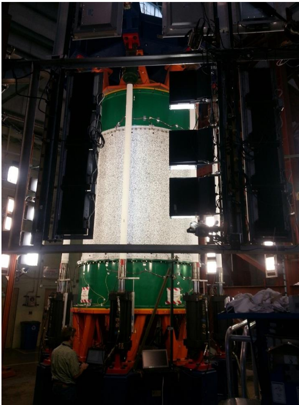
Composite Shell Buckling Test
