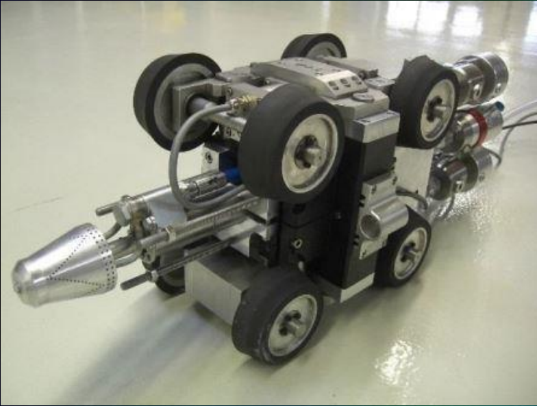
Internal Coating Robot with nano-circuit axial, circumferential and layer positional encoding
